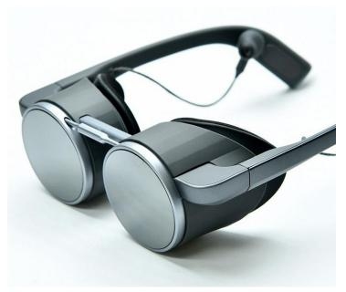
**Panasonic** launched the world's first high dynamic range (HDR) VR glasses. The technology enables high-definition, quality content to be viewed in a compact, lightweight design. The company worked with 3M and Kopin Corporation to develop an optical module that enables distortion-free and natural image viewing in a single focus.
