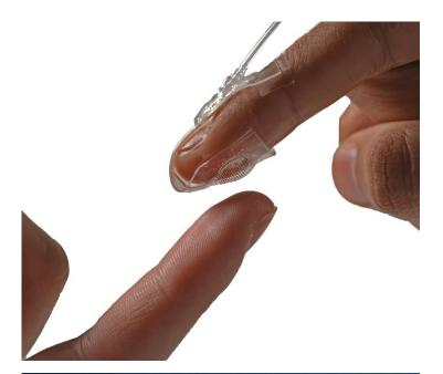
Researchers from the Swiss Federal Institute of Technology revealed a portable interface that allows VR users to feel objects in virtual environments. The silicone-like, electrode-like skin supplement is packed with sensors and activators that work together to realistically mimic the sense of touch. The prototype is limited to a finger device; however, more applications are expected in the future.
