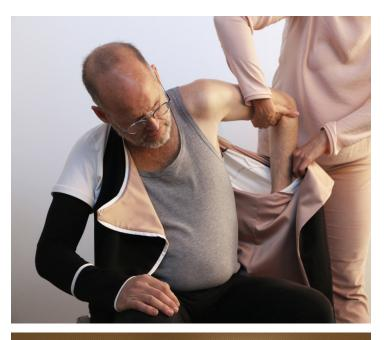
Jessica Smarsch, founder of the startup **Constructing Connectivity**, developed Connextyle, a wearable-shaped shirt that has 'technical sleeves' lined with sensors that measure muscle activity, joint rotation and are linked to a mobile app that visually tracks progress, helping patients who have suffered from a stroke regain muscle function.
